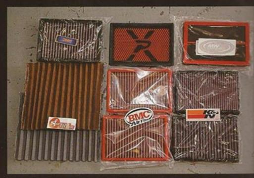
So the trio put together an air filter test, gathering various aftermarket elements from MWR, Sprint, K&N, Pipercross, DNA and BMC. Max air flow testing was carried out at the university using the clever equipment and facilities they have at their disposal, before getting properly technical and analysing samples of each filter under the microscope to understand design and structure. The final slice of the test involved using engine simulation software.
